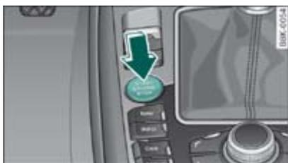
**Fig. 1** advanced key: Tecla START ENGINE STOP
